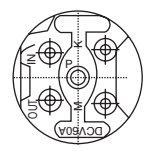
E2或E7 带测压口G1/4 (标准结构) with testing port G1/4 (standard)
